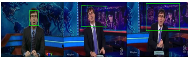
Fig. 8. Unexpected increase in the window size observed for the subsequent frames whose window is initialized by Viola-Jones. Later on discovered that this increase in window size is subject to deviation of mean from the expected due to background pixels inside the window.
