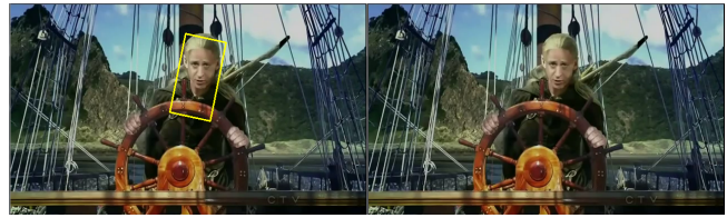
Fig. 9. Comparison of results generated by algorithm for compression ratio of 2:1 and 3:1 respectively. It can be noted that for lesser compression higher detection is observed.
