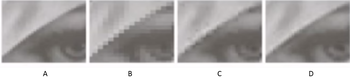
Figure 2: Applying DCT over left most image and reconstructing image with 25% of the coefficients.(a)original image (b) 2x2 block size (c) 4x4 block size (d) 8x8 block size
